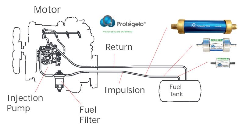
Preferably, the device is installed in the impulsion tube (before the filter).
